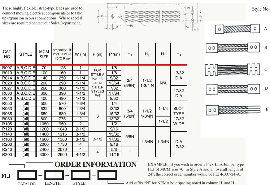
If you desire to use higher ampacities than shown DO NOT exceed a conductor temperature of 80°C (176°F) or approx. 120% of ampacities shown.
